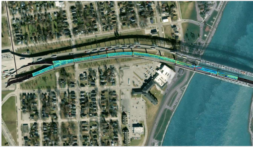
Google Earth View of Bridge Deck with GPR Scan Results
