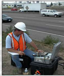
UPV test data recorded for pulse velocity arrival time analyses on Freedom NDT PC
