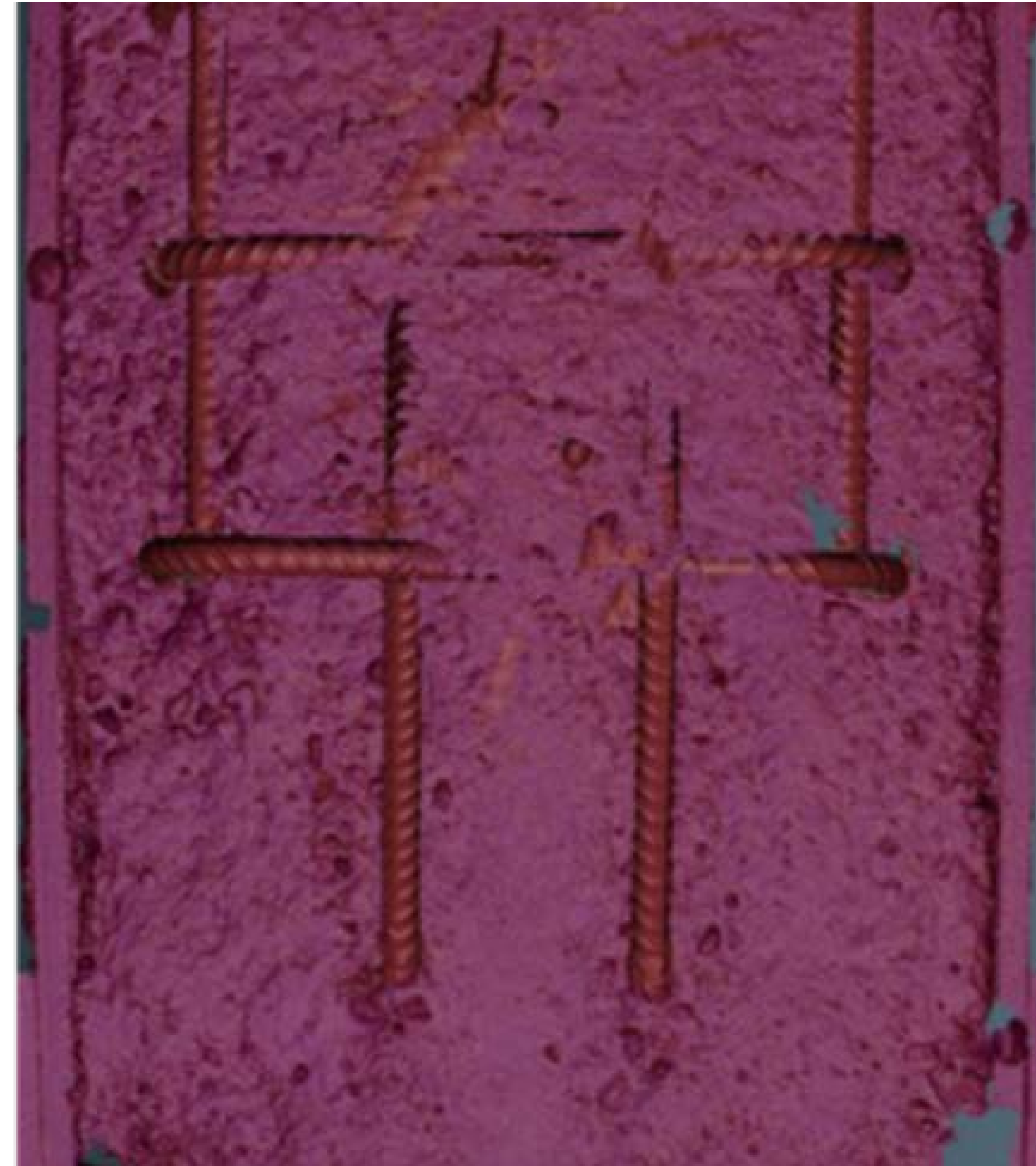
Photograph and laser scan of WJE Specimen 3 (As-placed)
