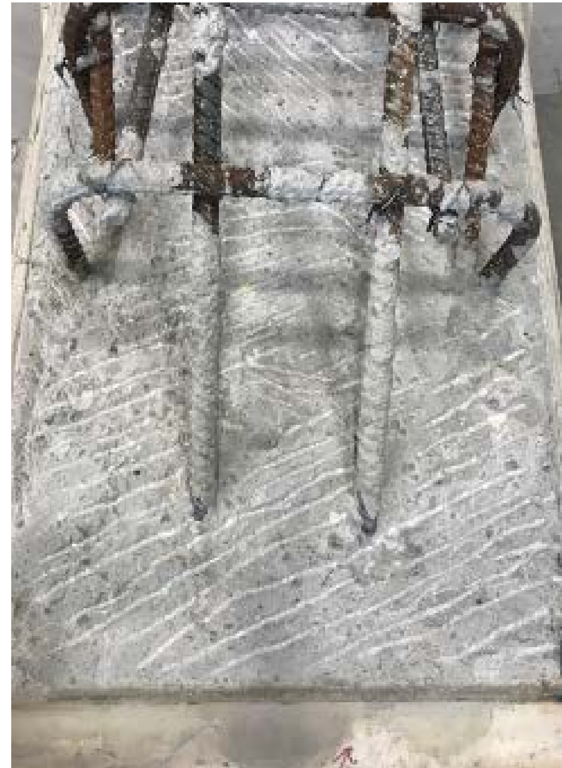
Photograph and laser scan of WJE Specimen 4 (Roughened)
