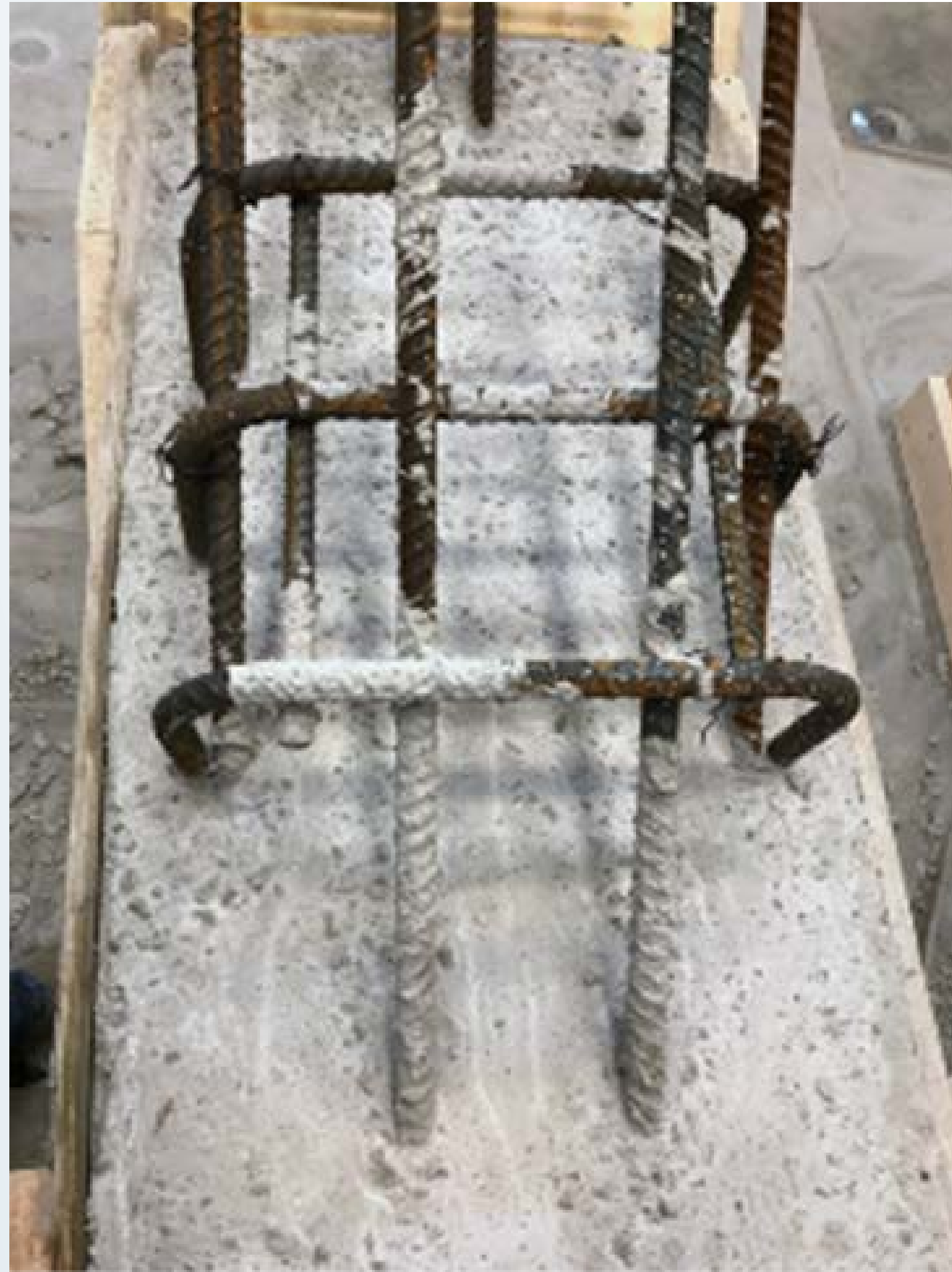
Photograph and laser scan of WJE Specimen 3 (As-placed)
