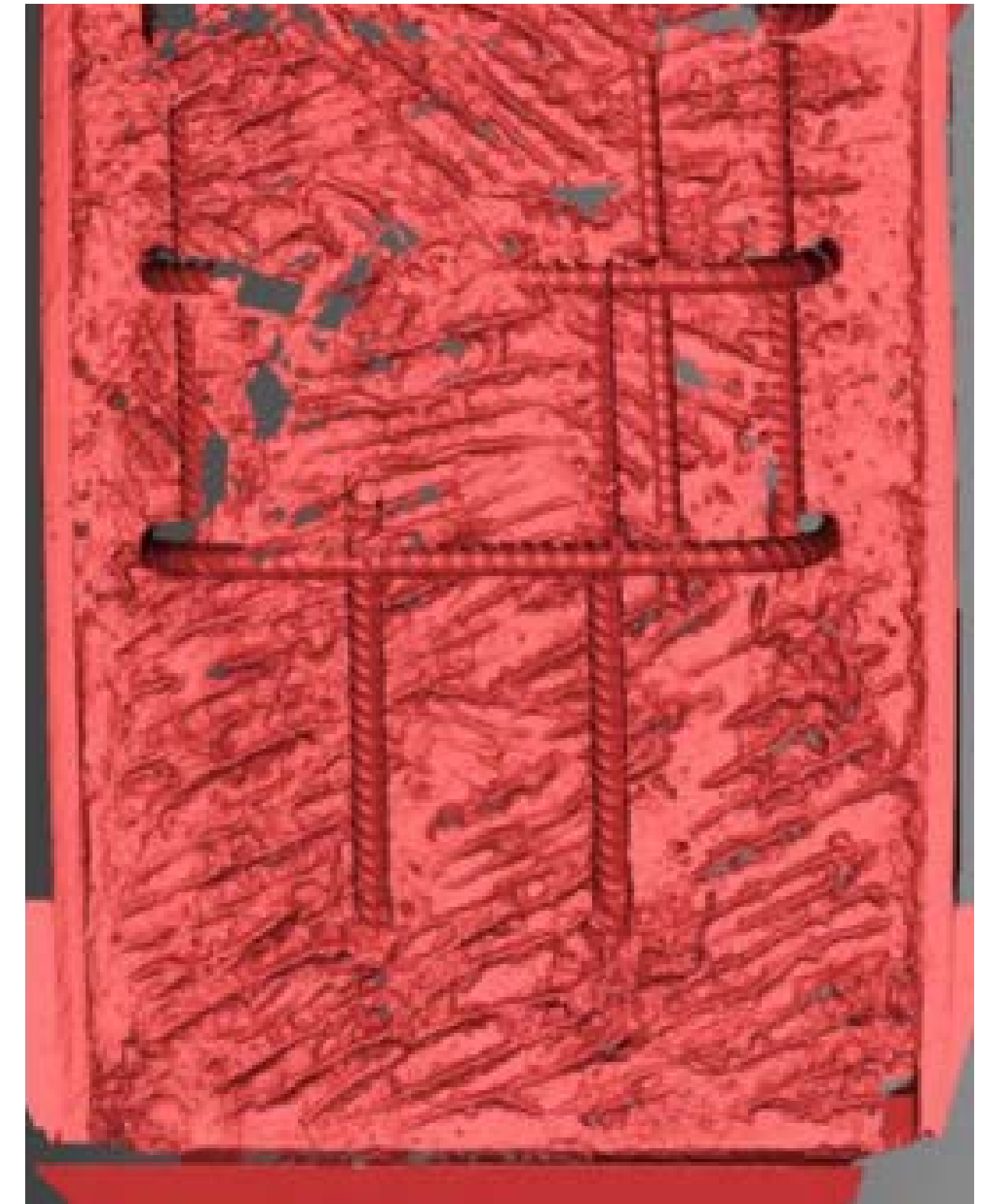
Photograph and laser scan of WJE Specimen 4 (Roughened)
