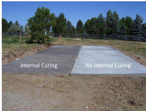
No conventional curing
