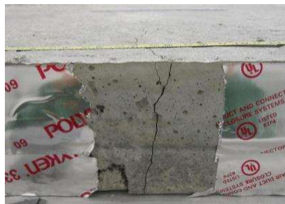
Plain 0.30 Concrete 0.6 mm wide crack observed @ 12 days
