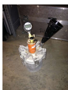
Shotgun: Funnel that attaches to the petcock
