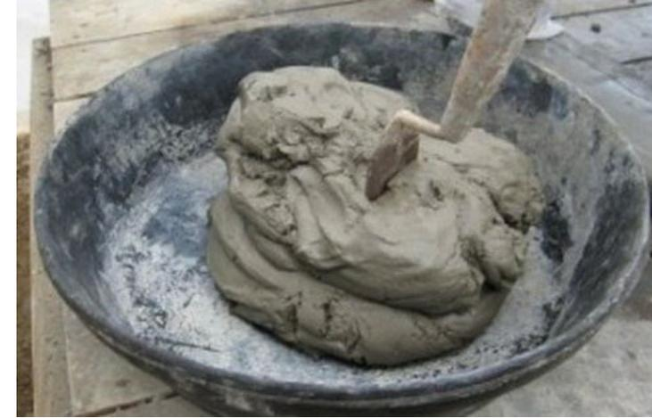
When water and cement meet they react and form a **paste** that glues the aggregate together.
