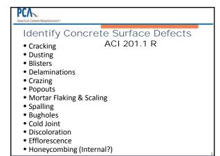
When troubleshooting concrete problems it is important to relate the symptom to causes of distress and deterioration.
